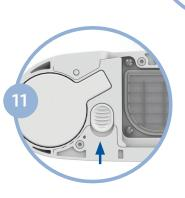
Insert column into the Inogen One<sup>®</sup> G<sub>3</sub> concentrator. Do not leave the column exposed; it should be inserted into the Inogen One<sup>®</sup> G<sub>3</sub> as soon as the dust caps have been removed.
