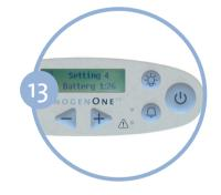
Press and hold the light button for 10 seconds and screen will display "sieve reset". Release button once message is displayed on screen. Press the bell button once and screen will display "sieve reset successful". Press the power button to turn on the Inogen One® G<sub>3</sub>, and use normally.
