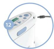
Connect the AC power supply cord to the Inogen One<sup>®</sup> G<sub>3</sub> and plug the power supply AC cord into an electrical outlet. **Do Not Power ON the Inogen One<sup>®</sup> G<sub>3</sub> concentrator.**
